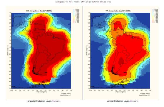
2.17 Horizontal (left) and vertical (right) availability obtained in SACCSA on 31/07/2012, with the network of stations used in SACCSA.
